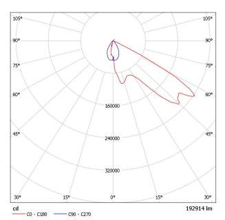
Luminaire classification according to CIE: 100 CIE flux code: 44 91 100 100 100
